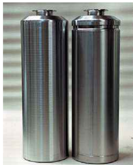
Containers for vitrified waste (left) and compacted waste (right).
