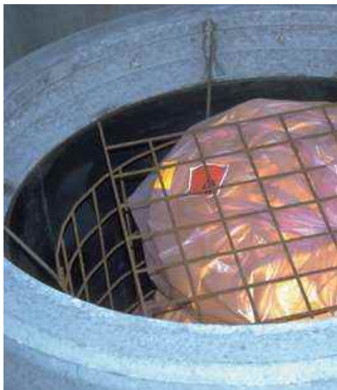
Solid waste in cemented drums before being embedded in cement.
