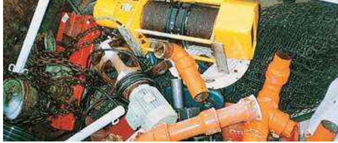
VLLW comprises rubble, scrap metal and piping, primarily from decommissioned nuclear facilities.
