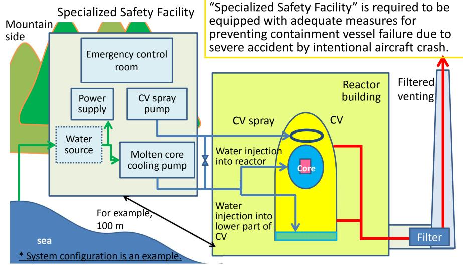
For BWR, one filtered venting for prevention of containment failure and another filtered venting of Specialized Safety Facility are acceptable solution.
