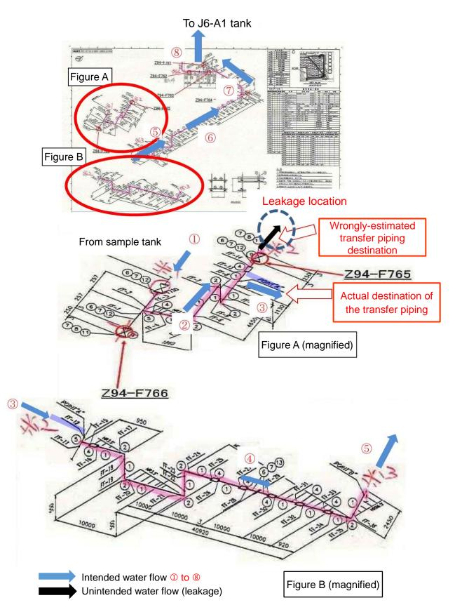
Figure 5. Treated-water transfer route map used during the preparation of the treated-water transfer manual\*<sup>7</sup>
