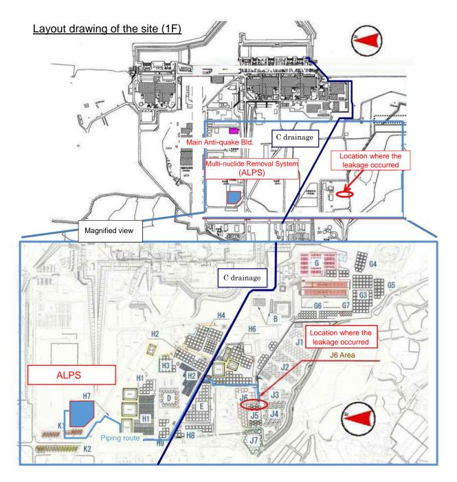
Figure 1. Layout drawing of J6 tank area \*<sup>3</sup> \*<sup>3</sup>: Excerpt from a TEPCO report (partially revised)
