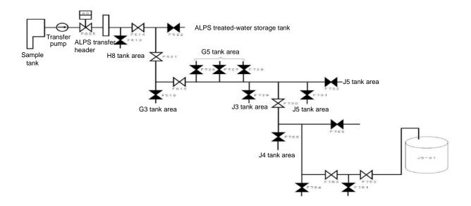
Locking and labeling of gate valves leading to piping under construction
