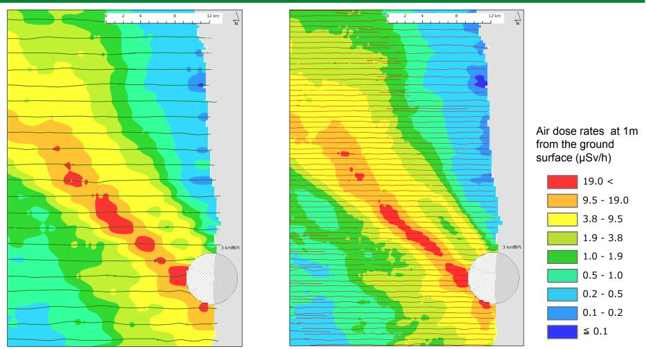
In the survey 30 months after the accident, the intervals of flight tracks were narrower comparing with the previous flight ones. It has created the map (right figure) with high resolution enough to figure out the distribution of air dose rates.
