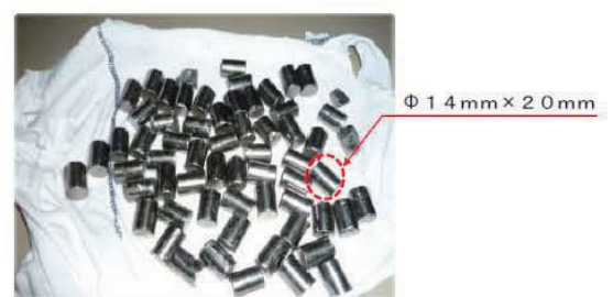
Photograph of the damaged bearing(roller)
