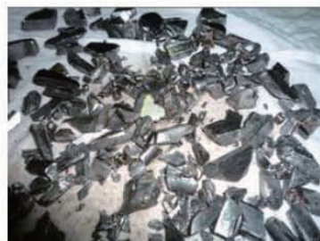
Photograph of the damaged bearing(inner and outer rings)
