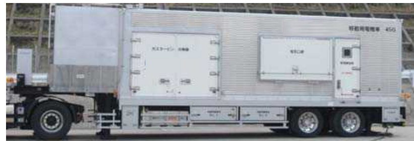
Alternative onsite AC power (Power Vehicle)
