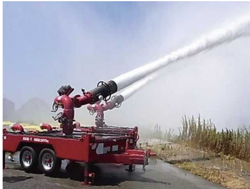
Water-spraying training with a large scale bubble water cannon system (Osaka and Wakayama wide area cooperative disaster prevention committee)
