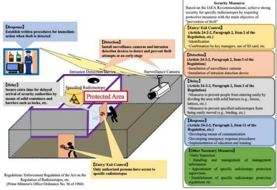
Figure 3-2: Protection Measures for Specific Radioisotopes
