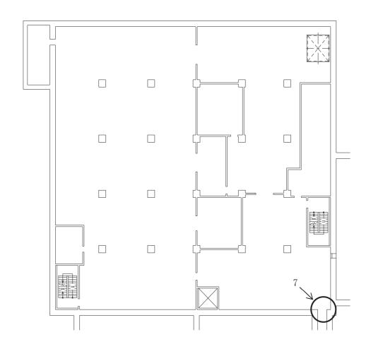
7 計測制御電源室(B)浸水防止水密扉(No. 3)
