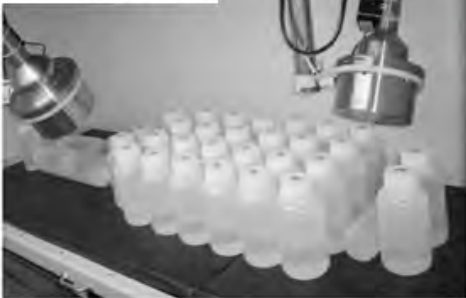
Figure 5.3: Bottle phantom (70-kg-configuration) in the WBC.
