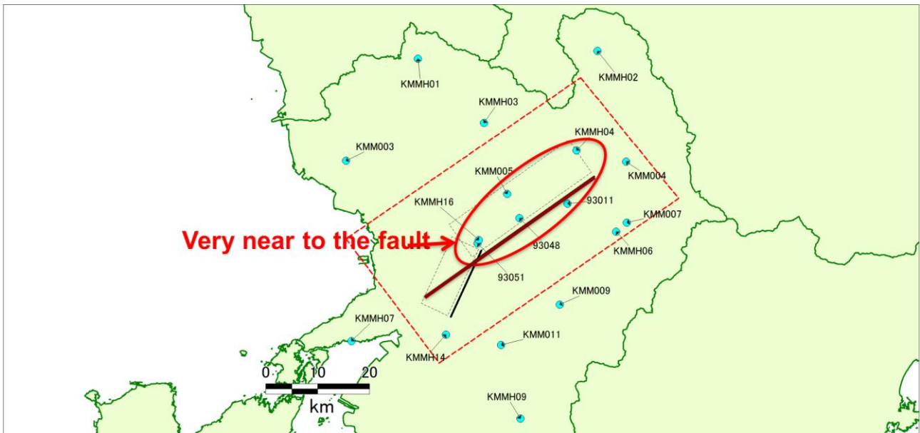
Figure 11. Map of station location (blue circle) for ground motion comparison and fault trace on surface of simplified fault model (solid red line). Stations inside the red dashed rectangle are near fault. Stations inside the rounded red line are considered very near to the fault. Rectangles with black dashed line represent projection of the actual faults of Futagawa (bigger rectangle) and Hinagu (smaller rectangle)
