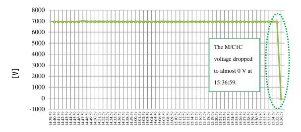
Figure 2.5 Behavior of M/C1C Voltage Value
