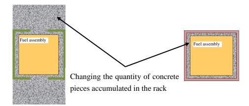
Figure 6.12 Evaluation Model with Change of Concrete Pieces Accumulated in the Rack
