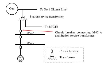
Figure 2.10 Overview of Electrical Connections for M/C1A and Station Service Transformer
