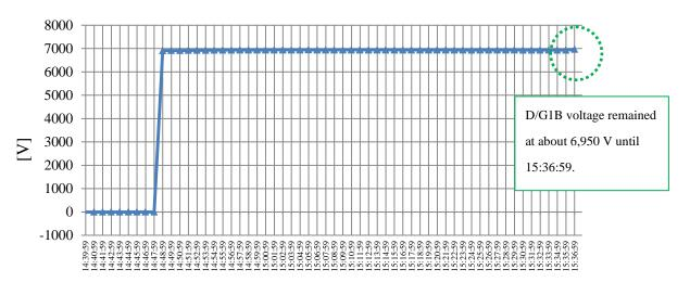
D/G1B voltage remained at about 6,950 V until 15:36:59 (Fig. 2.6). M/C1D voltage connected to D/G1B also remained at about 6,950 V and was ready to supply power until 15:36:59 (Fig. 2.7).
