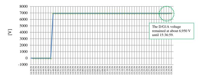
Figure 2.4 Behavior of D/G1A Voltage Value
