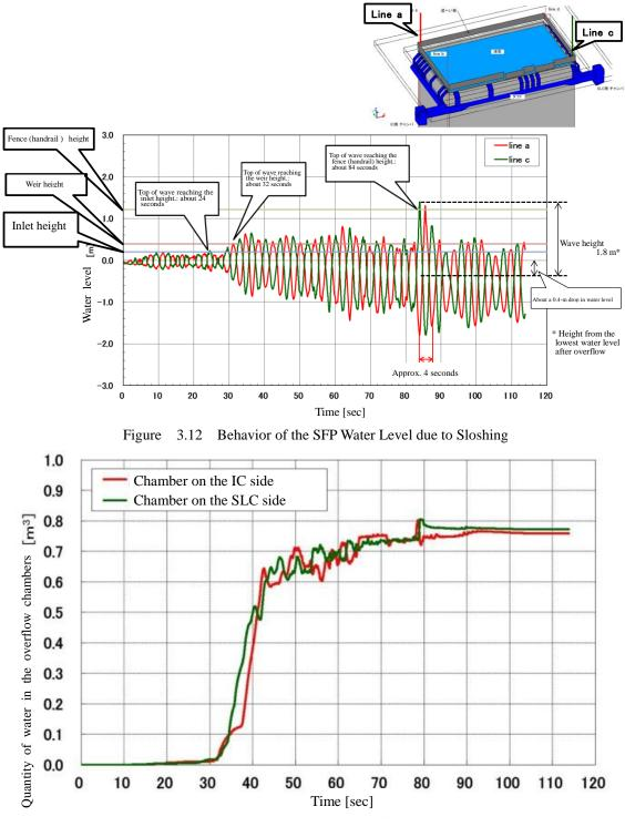
Figure 3.13 Behavior of Water Quantity in the Overflow Chambers
