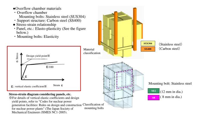
Figure 3.16 Overflow Chamber Deformation Evaluation Conditions (2)
