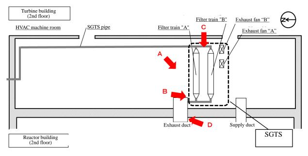
Figure 7.7 Layout of the SGTS Filter Trains, etc.
