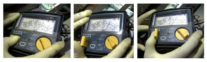
$2.8 \text{ M}\Omega \text{ between R and S phases } 1.9 \text{ M}\Omega \text{ between S and T phases } 2.7 \text{ M}\Omega \text{ between T and R phases } \\ Figure \ 2.15 \text{ Measured Interphase Insulating Resistances } Photographed by the NRA on June 5, 2014. } \\$
