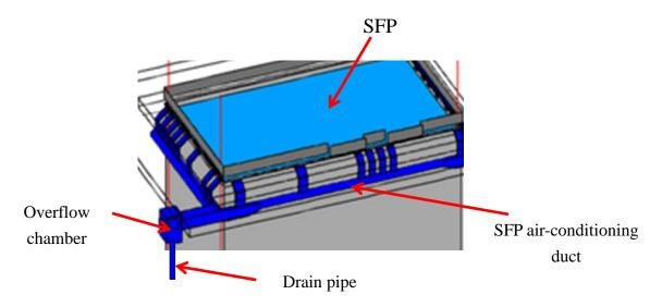
Figure 3.5 Location of the SFP, SFP duct, and Overflow Chamber (image diagram)
