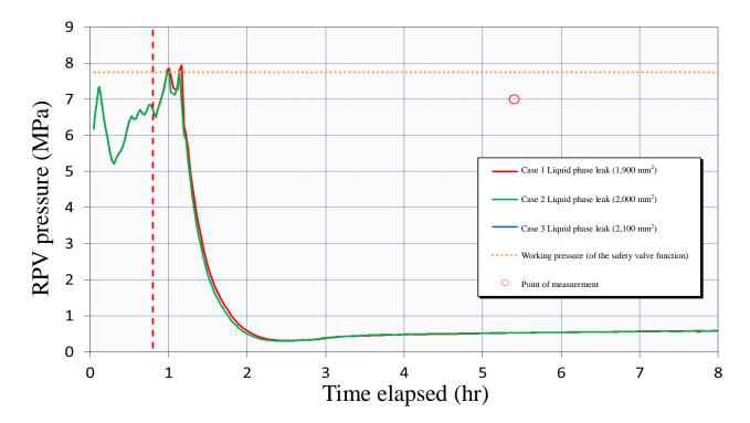
Figure 4.4 Behavior of RPV Pressure (cases with leak from the liquid phase) The solid line indicates the analysis result; "o" indicates the measured pressure value.
