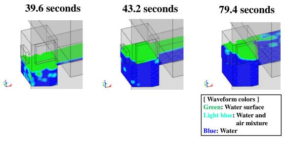
Figure 3.14 Water Flow into the Overflow Chambers (analysis result)
