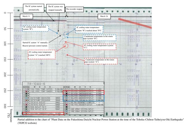
Figure 5.9 IC System-related Temperatures in Unit 1
