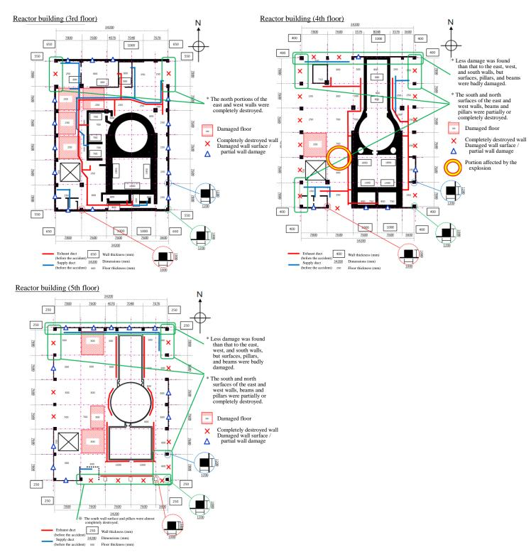
Figure 7.15 Traces of Damages on the Reactor Building (floor, ceiling, and walls)
