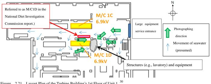
Figure 2.21 Layout Plan of the Turbine Building's 1st Floor of Unit 1
