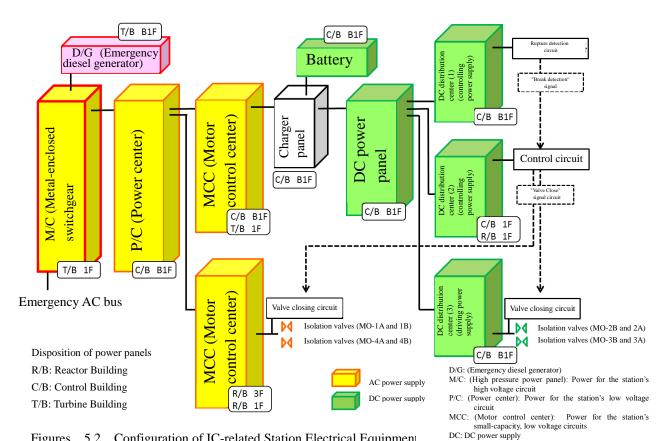
Figures 5.2 Configuration of IC-related Station Electrical Equipment
