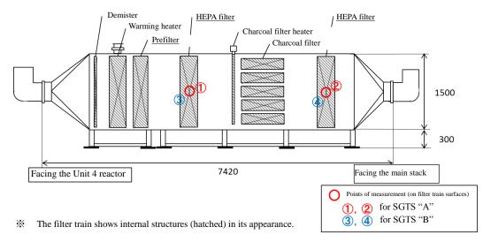
Figure 7.3 Structure of the SGTS Filter Train
