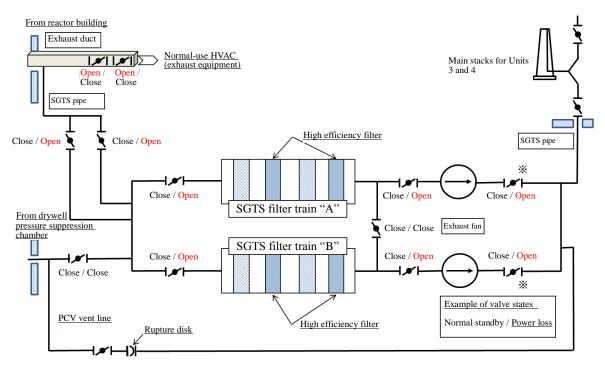
Figure 7.1 Block Diagram of the SGTS of Unit 4 (overview)
