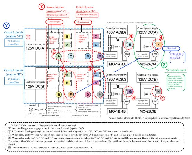
Figure 5.8 IC Isolation Valve Working Mechanism in case of Controlling Power Loss (operation logic "B")
