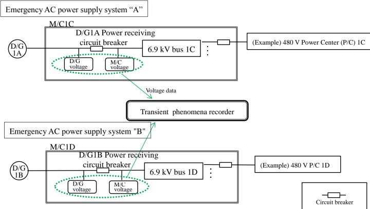
Figure 2.2 Outline of Power Supplies to Transient Phenomena Recorder and Data Collecting Positions
