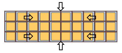
(Case b) Criticality analyses model (moving fuel assemblies toward the center of a boron-added aluminum rack)Figure 6.8 Criticality Analyses Models of Fuel Assemblies Compaction towards the Rack Center
