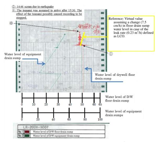
Figure 1.3 Water Levels of Drywell Floor Drain Sumps and Equipment Drain Sumps <sup>5</sup>
