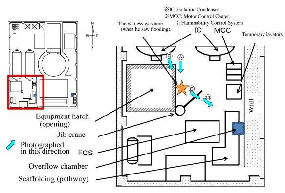
Figure 3.2 Standing Position of Witness when Water Leak came out
