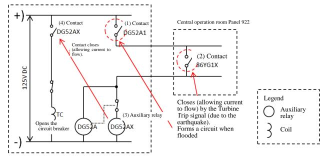
Figure 2.18 D/G1A Control Circuit Diagram
