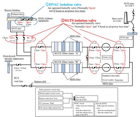
Figure 7.18 Logic of Starting Normal-use HVAC System and the SGTS in the Reactor Building of Unit 4
