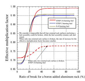
Figure 6.15 Characteristics of the Effective Multiplication Factors in terms of Rack Deformation and Break
