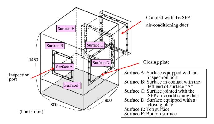
Figure 3.7 Structure of the Overflow Chamber (image diagram)
