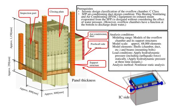
Figure 3.15 Overflow Chamber Deformation Evaluation Conditions (1)
