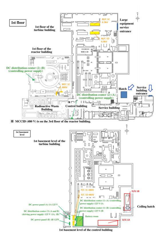
Figure 5.4 Layout of IC-related Station Electrical Equipment (on the 1st floor and 1st basement level)
