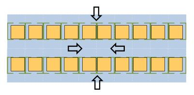
(a) Criticality analyses model (moving fuel assemblies toward the center of an aluminum rack)
