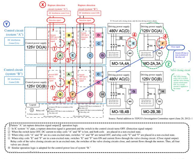
Figure 5.7 IC Isolation Valve Working Mechanism in case of Rupture Detection Signal Generation (operation logic "A")
