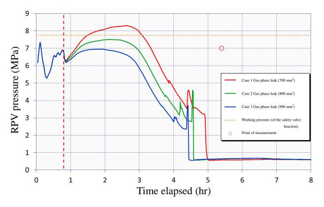
Figure 4.3 Behavior of RPV Pressure (cases with leak from the gas phase) The solid line indicates the analysis result; "o" indicates the measured pressure value.
