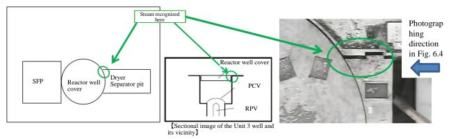
Figure 6.6 Equipment Layout on the Top of the Reactor Building of Unit 3 Source: TEPCO documents edited by the NRA (and photos taken by TEPCO on January 31, 2014)
