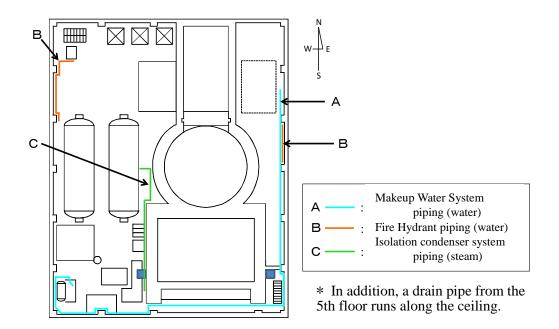
Figure 3.4 Water and Steam Pipes installed on the 4th Floor of the Reactor Building of Unit 1
