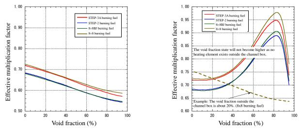
(a) Change of the void fraction only inside the channel box
