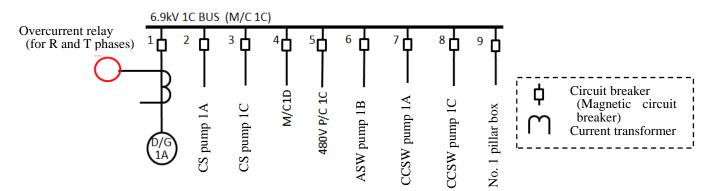
Figure 2.11 Electrical Connections for M/C1C and the Locations of Overcurrent Relays
