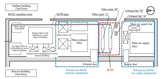
Figure 7.5 Layout of the Normal-use HVAC System and the SGTS
