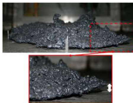
Figure 40: The melt spread in PULMS-E1 experiment (side view). The volatile particle debris have been removed while solidified core of the melt remained intact.
