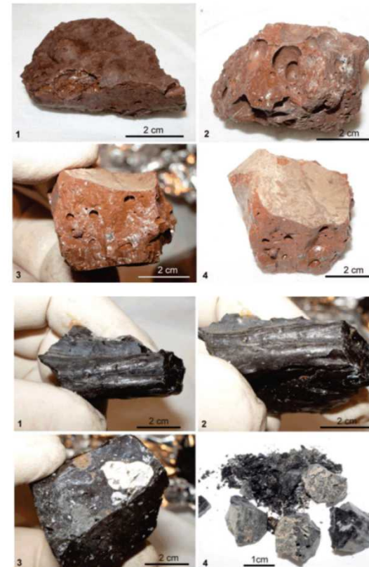
Figure 2.5-3: Corium samples (TOP 1-4: brown ceramic from the large vertical flow; BOTTOM 1-4: black ceramic from room 304/3) (Burakov, 2013)
