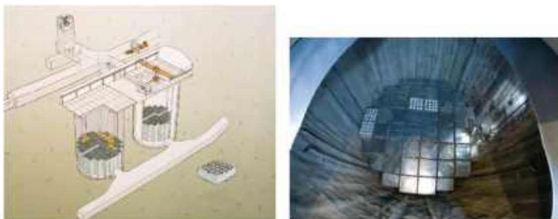
Figure 8. The Olkiluoto LLW repository. LLW drums in the disposal silo (left) and cross-sectional view of the repository lay-out (right).
